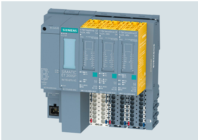
SIMATIC ET200SP 的驱动模块 SIMATIC MICRO-DRIVE F-TM StepDrive ST、ServoDrive HF 和 ServoDrive ST
